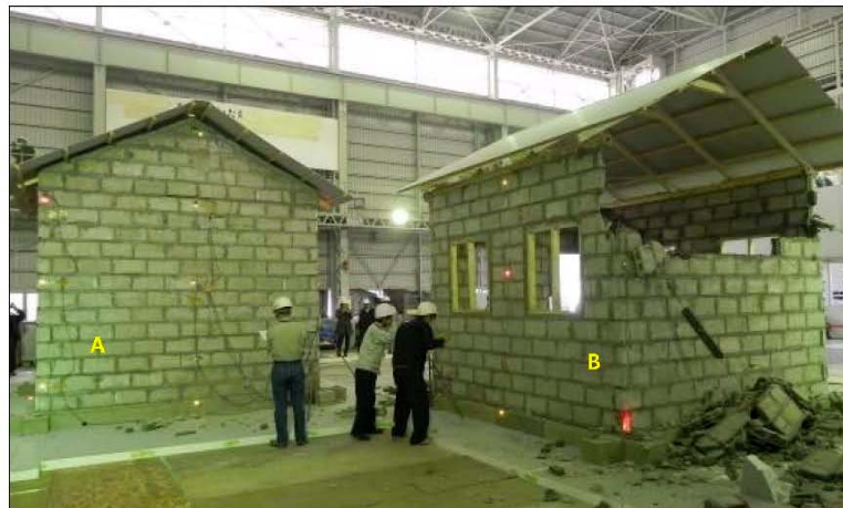
Picture shows the collapsed gable part of the back wall of model B
